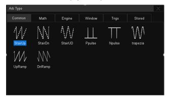
The USB waveform generator can output waveforms with up to 25 MHz frequency and ±3 V amplitude. Six basic waveforms together with multiple types of predefined waveforms and as user-defined arbitrary waveforms are supported.
