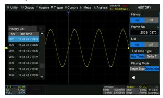
History function can record up to 80,000 frames of waveforms. The recording is executed automatically so that the customer can playback the history waveforms at any time to observe unusual events and quickly locate the area of interest using the cursors or measurements.
